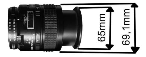
These are precise dimensions. To determine "**d**", I need to add a bit more to these 65mm so that I can insert the moving part in it, but it MUST be smaller than 69mm so that I can sit my lens on its fixed surface. To determine "**D**", it needs to be slightly bigger than 69,1mm.
