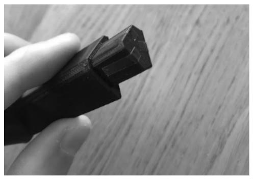
Now that the BODY assembly should be dried (verify the glue had enough time to dry before continuing), we will assemble the arms on it. Simply remove the protective layer of each double sided tape strip and slide the arms until they stop. The double sided adhesive will create some friction, and this is good. To secure the assembly, I am using electric tape and make two or three well tight turns around each junction.
